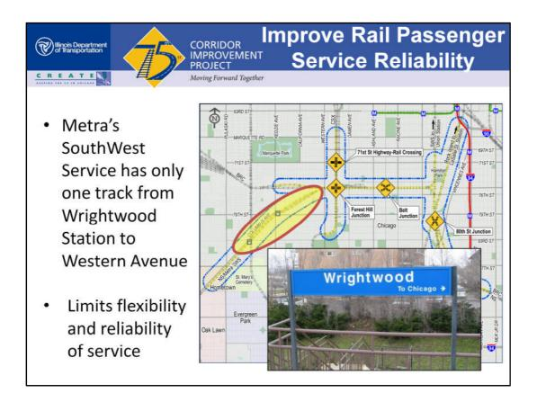
From Wrightwood Station to Western Avenue, Metra operates on a single track, but Metra runs on double track east and west of there. Since the Metra trains run in both directions, one train is sometimes delayed while the other one clears the single-track segment. This can cause service delays and less reliable transit service. A second track in this area will allow Metra to run trains in both directions throughout the corridor.
